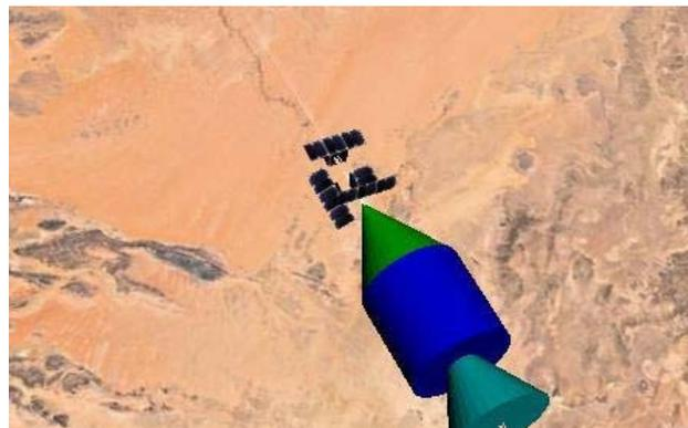
Fig. 2 View of the formation in Earth coordinates after release from upper stage. Formation deployment start with one satellite slowing down and another veering off-plane.
