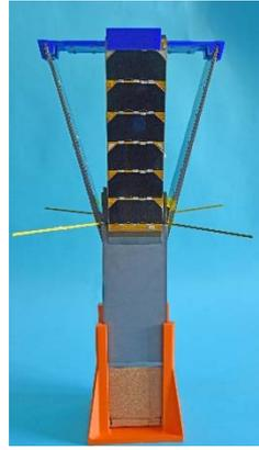
Figure 2: QARMAN flight model in deployed configuration.
